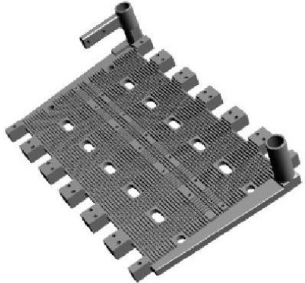
Test of a 3D-printed cooling plate for a TPC using 2-phase CO2 By university Paris Sacry and DESY
