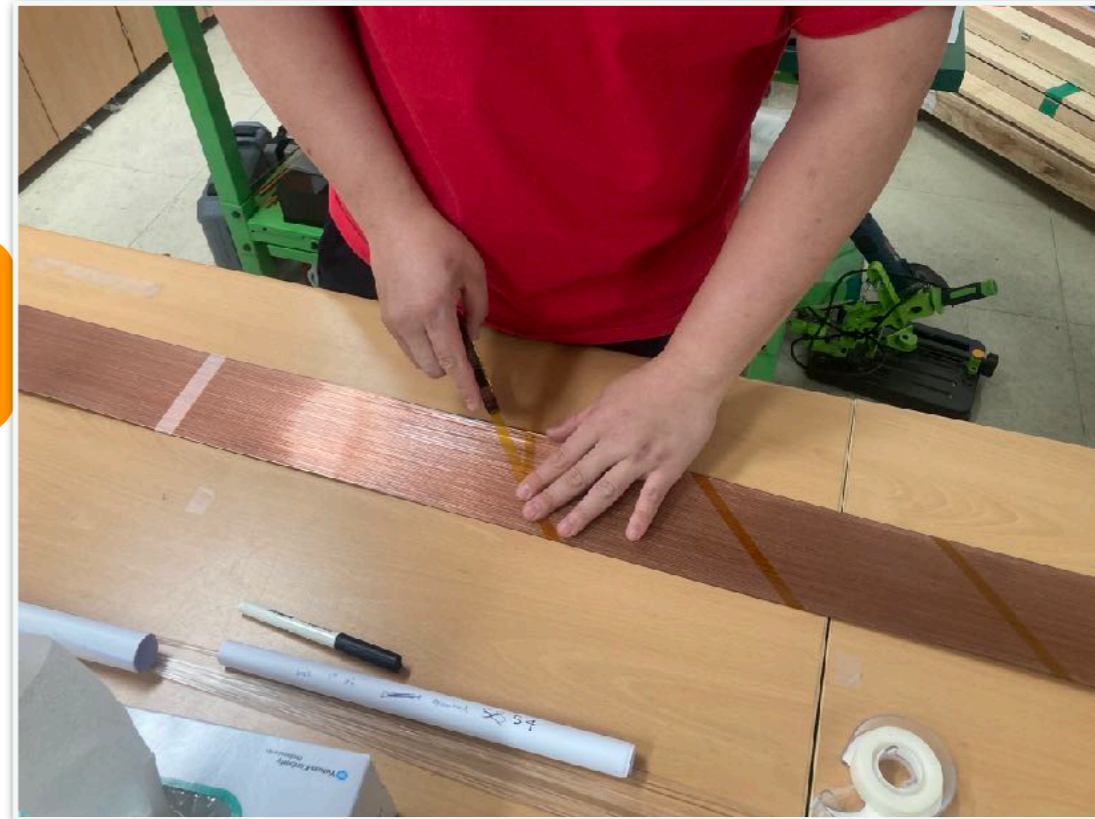
alignment, taping, and painting scintillating fibers
