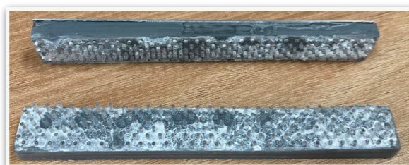
Removed čerenkov holders
