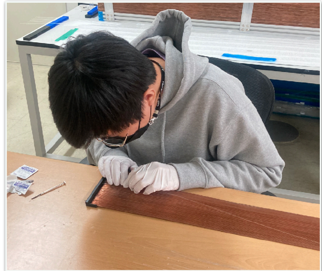
alignment, taping, and painting scintillating fibers
