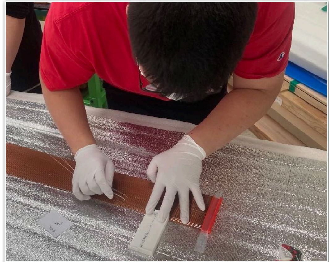
alignment, taping, and painting scintillating fibers
