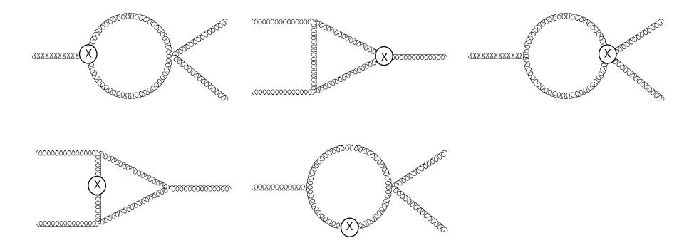
There are five diagrams contributing to the renormalization for each operators.  $\bigotimes$  means the inserted operator with zero momentum.
